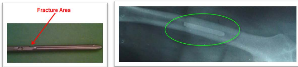
Figure 2: Image of SP2 IM Rod highlighting area of potential fracture / Image of SP2 IM Rod fragment in a radiograph
